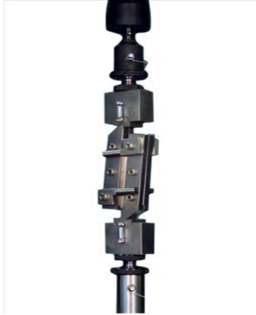
Figure 3.21 Two-rail shear test
